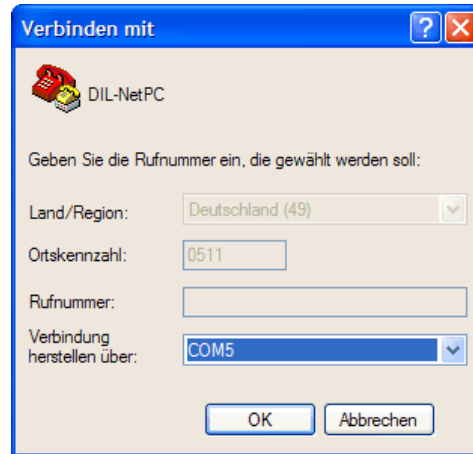
Figure 5: Direct connection setup with HyperTerminal
